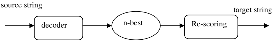
Fig. 1. The decoding illustration of our phrase-based translation system
